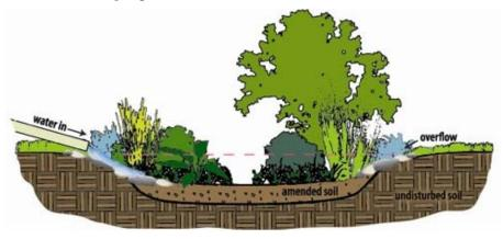
This vegetated infiltration basin in the field at the corner of Swanton and Niantic Avenue will help prevent polluted stormwater run-off from the neighborhood from reaching Mashapaug Pond. The stormwater will flow to a rain garden and soak through permeable soils into the groundwater.
